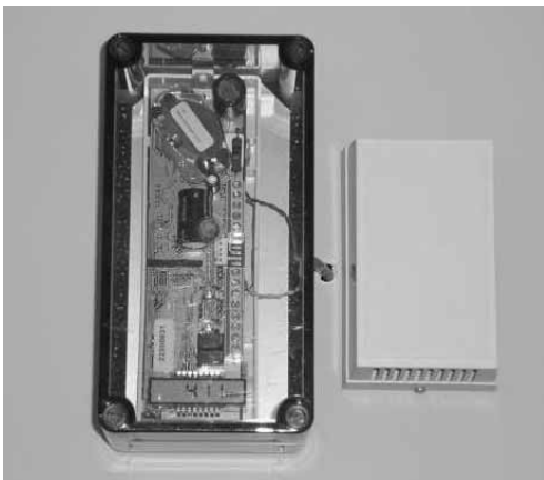
Figure 5: Air quality monitoring device measuring CO 2 and CO
