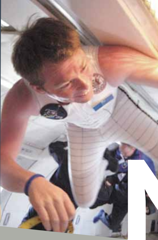
Dr James Waldie flew on a zero-gravity aircraft to test the comfort, mobility and material properties of his skinsuit.
