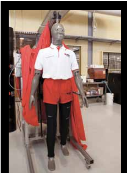
A thermal mannequin will enable researchers to study the response of human skin to different textiles
