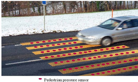
Fig. 1. A proposal for an instrumented pedestrian crossing
